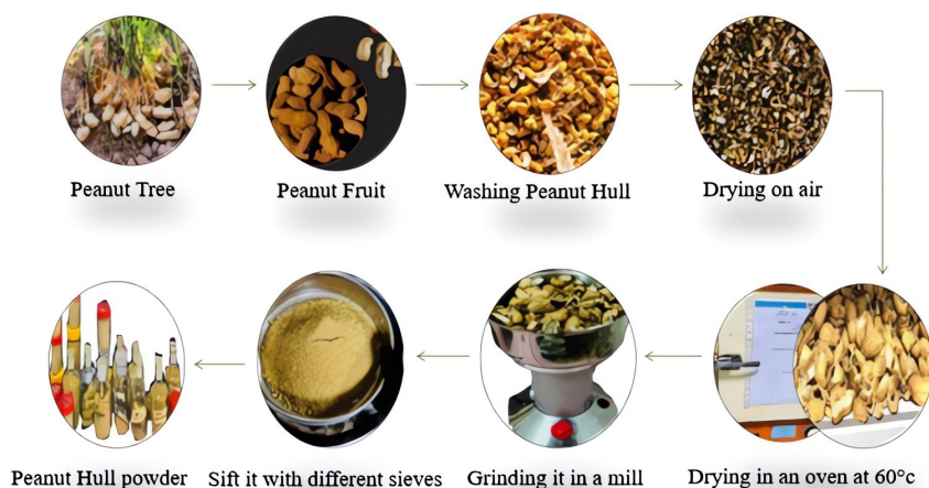
Fig. 1. Preparation of Peanut Hull Powder for Adsorption Experiments
