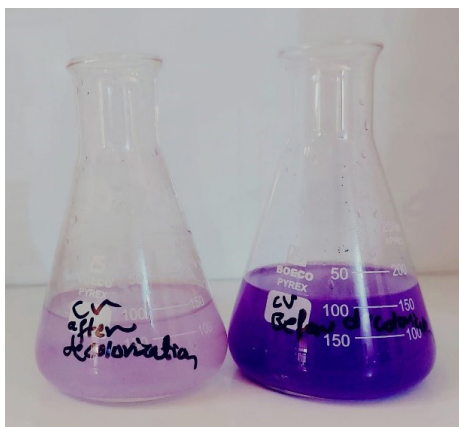
Fig. 10. Aqueous Solutions Containing Crystal Violet Dye before and after Adsorption Process by PHP
